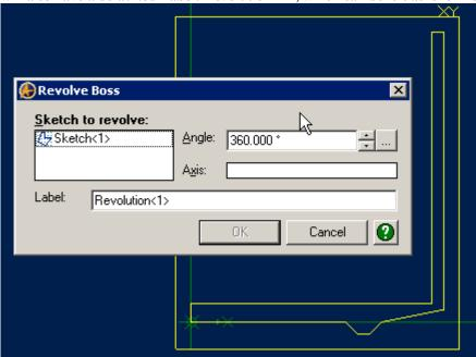
Only remaining item to select is the  $A\underline{x}$  is: Click in the space for Axis: Then select the Y-axis, the vertical green line in the sketch (Y-Axis), As you mouse over it, it will become Red:
