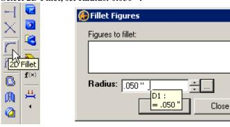
Select the bottom line extending right from the origin (Line<1>), and the first 45 degree Line down (Line<2>),
