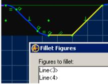
Select the second 45 degree line (Line<4>), and the next up-sloping line (Line<5>), Click Apply.
