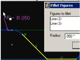
Select the bottom Line (Line<3>), and the second 45 degree line (Line<4>), Click Apply.
