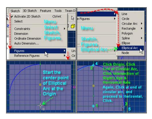
Again, click the end of the Circular Arc, and drag down to the right to begin tracing how far the Elliptical arc will cover, stopping at the Horizontal. Click to end.
