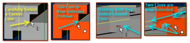
• You may need to rotate the view of the extrusion around to get both, remember to shift-click.
